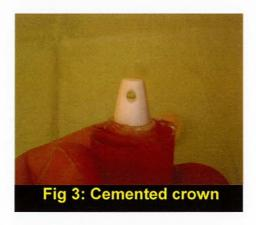
Specimens of <u>Group1</u> were cemented with Temposil (experimental, Coltene/Whaledent) according to manufacturer's directions. Specimens of <u>Group 2</u> were cemented with Temposil (Coltene/Whaledent)following the manufacturer's directions. Specimens of <u>Group 3</u> were cemented with TempBond NE (Kerr)
